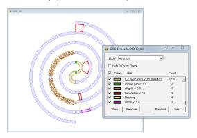
In addition to dw-2000's standard microelectronic checks, the program's ability to handle all-angle geometries makes it more flexible and capable of locating errors correctly in non-traditional designs. For example, checks can be optimized for curves and rounded shapes in order to avoid false positives and increase yield.
